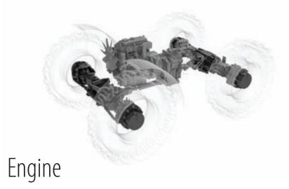
The ALPHA Series engine is one of the most economical and durable in its class. The turbocharged, 4.400 cm<sup>3</sup> engine maintains high torque even at low rpms.
